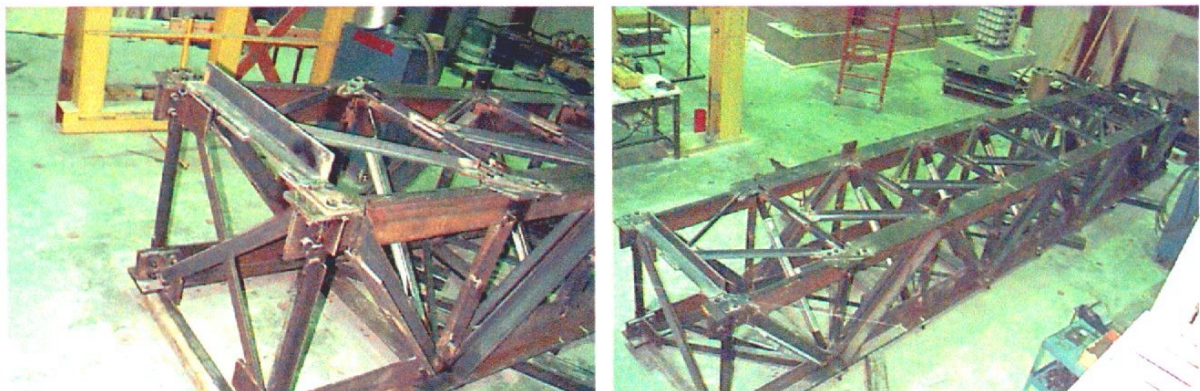
Figure 8: Deck-truss 1:10 model (without the ductile retrofit devices) during construction.
